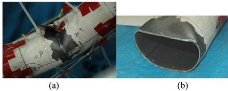
**Fig. 4.** Postbuckling behavior at the midpoint of specimens (Specimens 728 and 732): (a) local buckling ( $\epsilon_n = 2.0\%$  first cycle); (b) fracture section (after  $\epsilon_n = 2.0\%$  second cycle)
