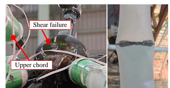
(c3) Bolt fracture (c4) Crack propagation
