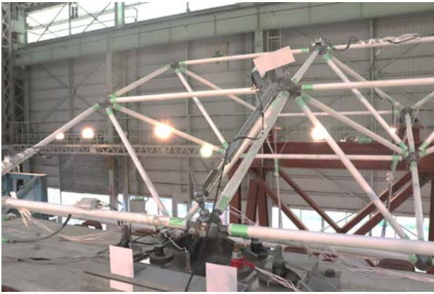
Figure 10: Measurement detail around the roller support
