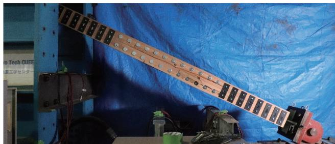
(L4) Out-of-plane failure (WpL)
