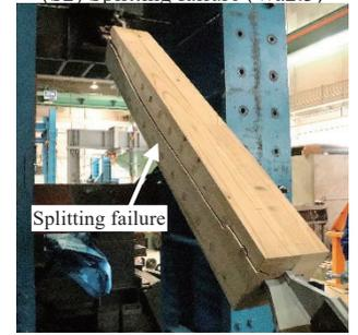
(S4) Splitting failure (Was)
