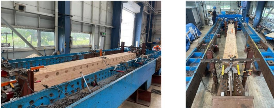
Fig. 22. Test setup for full-scale MT-BRBs.
